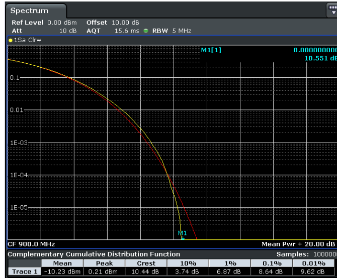
Fig. 76: CCDF of a 3GPP signal (yellow) compared to the noise (red).
