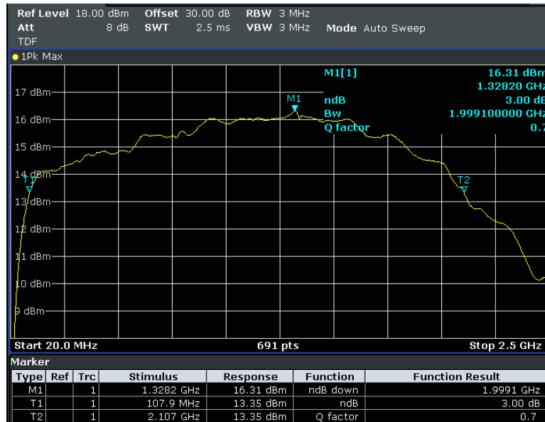
Fig. 46: Frequency response at an instantaneous amplitude for maximum power – 10 dB.
