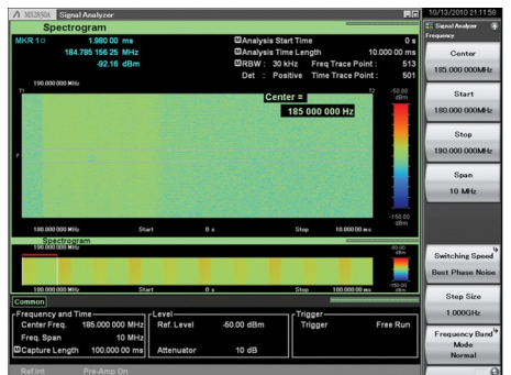
Figure 78 : Noise when LED lit
