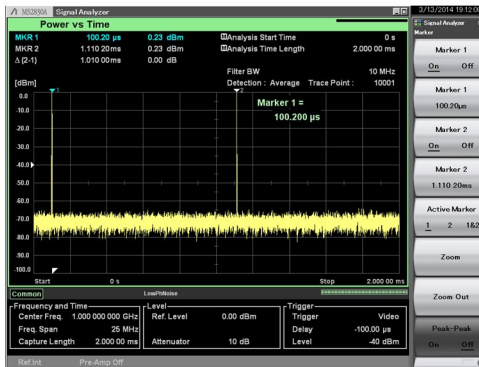
Figure 84: Measurement of 1 kHz Pulse Repetition Frequency in Power versus Time operation mode
