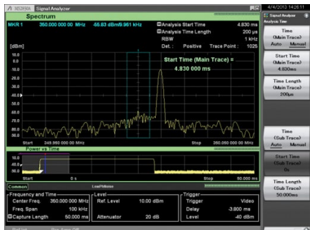
Figure 64: 2-FSK signal instantaneous Spectrum-1
