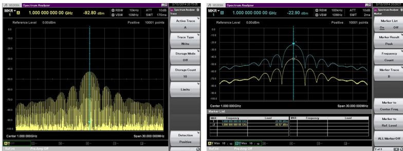
Figure 87: Pulse Spectrum for RBW of 10 kHz (left), 20 dB spectrum growth for 10 fold RBW (right)
