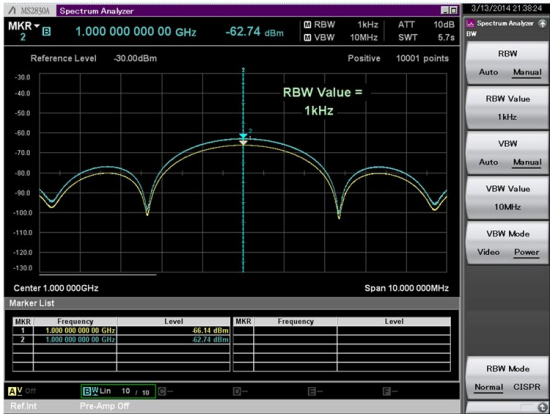
Figure 94: Signal under test measured with RBW 1000 kHz / VBW 10 MHz and 10 Hz and an average factor of 10
