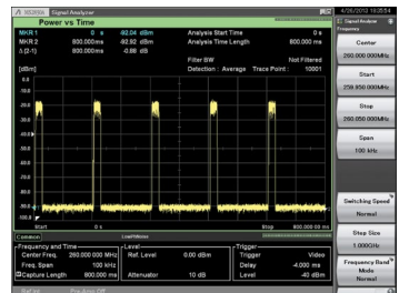
Figure 14: Example of Power vs. Time trace (ARIB T61 Emergency radio burst signal)
