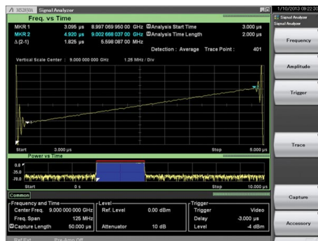
Figure 63: Split screen display of chirp signals (Main trace: Frequency vs. Time, Sub-trace: Power vs. Time)
