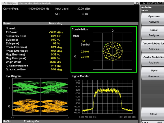
Figure 107: \pi/4 -DQPSK modulation with perfect interference free modulation and ~0% EVM
