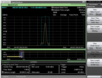
Figure 58: Spectrum transition immediately after Start-3
