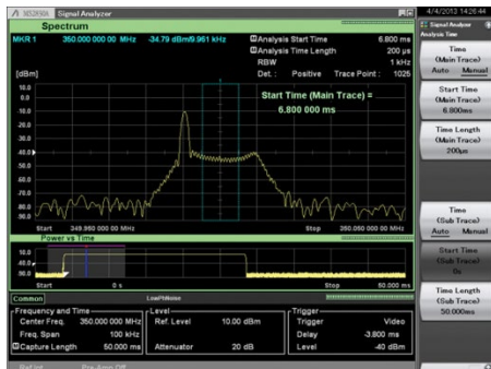
Figure 66: 2-FSK signal instantaneous Spectrum-3
