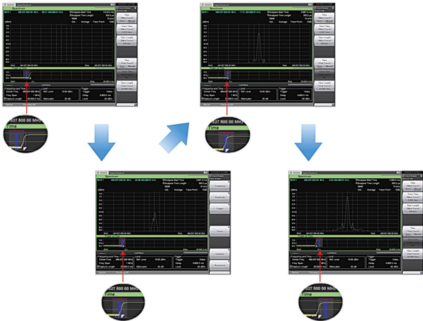
Figure 7: Sequential display of wireless signal spectrum display captured in memory
