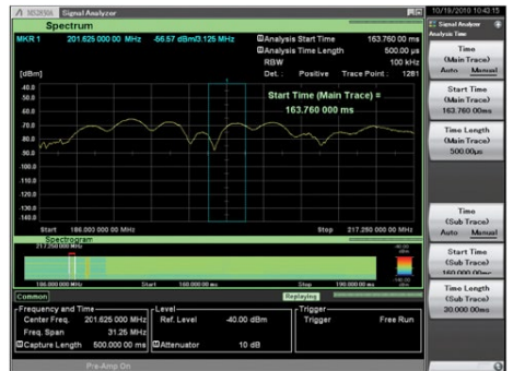
Figure 75: Instantaneous spectrum at power-on
