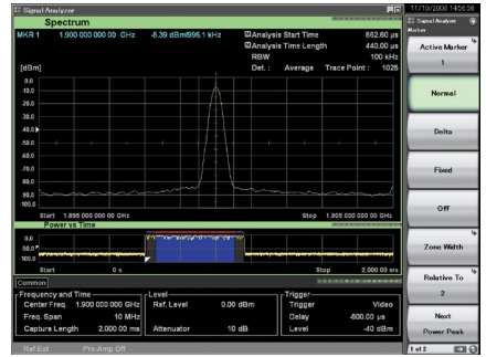
Figure 20: Example of split screen display (Main trace: Spectrum, Sub-trace: Power vs. Time)
